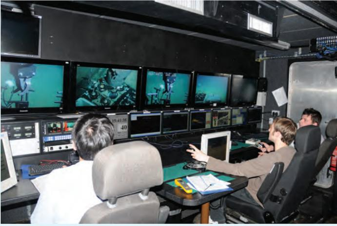
Back in the ROV control van, we are at the seabed and there are a series of checks. At 2500m the ROV is under 250 atmospheres of pressure. The ROV pilots check all the technical and recording equipment. The commands we give on the joystick are transmitted instantaneously to the ROV nearly two miles away.
